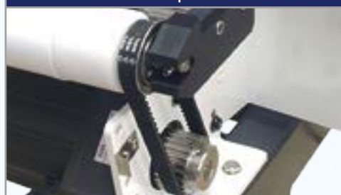
Timing belt never interfere transportation belt.
