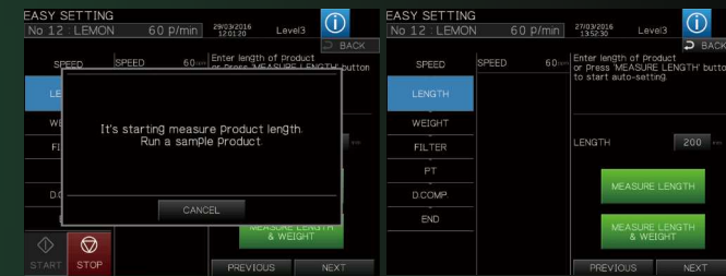
Product length is measured automatically Simple product type setting screen
