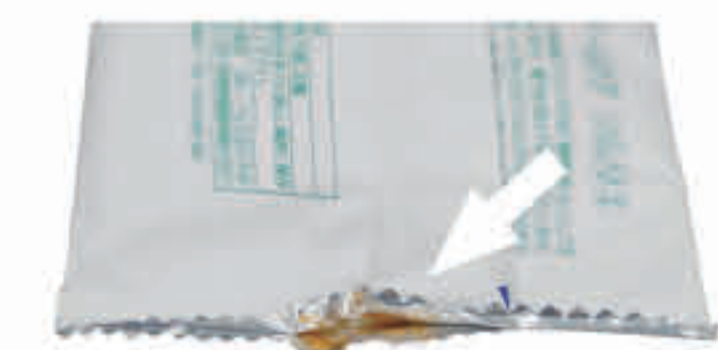
Example of failed seal
